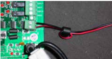
Ferrite sleeve on the power supply cable
