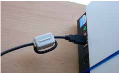
Folding core on the USB cable to the computer
