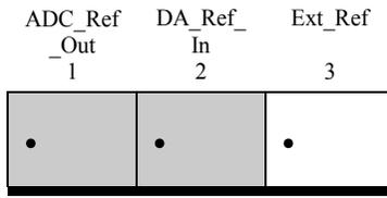
JP4 is used to select voltage reference source for DAC. When short pin 1 and pin 2 means select a default +5V as reference source for DAC, otherwise short pin 2 and pin 3 means select an adjusted +5V (which is adjustable using VR1) as reference source for DAC.
