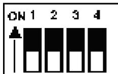
The S2 switch is used to identify USB card ID. Please set different card ID to each card (do not duplicate card ID setting).
