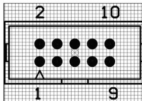
To use RS422/RS485/RS232, please connect J2 to extension board by 10 pins flat cable.
