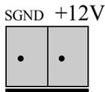
The power of USB 14/16 bit data acquisition board can be supplied from USB; however, if USB can not supply enough power, the external power is need. To input external power, please use the pin 1 and pin 2 connectors of TB2. Be careful to input DC +12V power.
