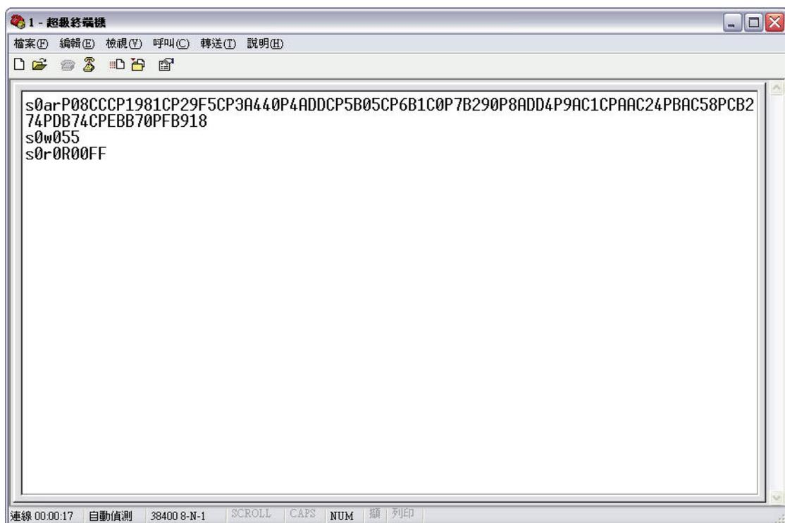
8. Or you may write a COM port communication program to operate the USB ADDA board. There is also an example VC program in the software directory called "USBtest\_hostxp\_vc\_110519ad\_beta".
