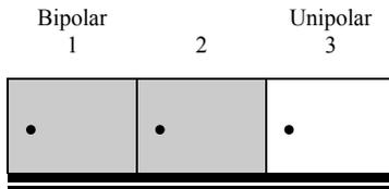
JP5 is used to select Bipolar/Unipolar of ADC converter range. When short pin 1 and pin 2 means select bipolar of ADC input, otherwise short pin 2 and pin 3 means select unipolar of ADC input.
