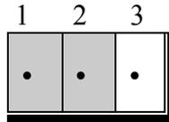
The MS1 is located at RS422/RS485 extension board. MS1 is used to set RS422/RS485 communication, when short pin 1 and pin 2, means set RS422. When short pin 2 and pin 3, means set RS485.
